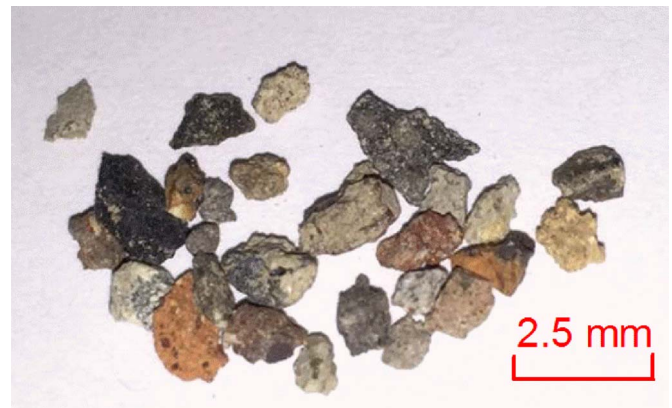
Fig. 2. Typical image of recycled concrete aggregate fraction 1.18–2.36 mm.
